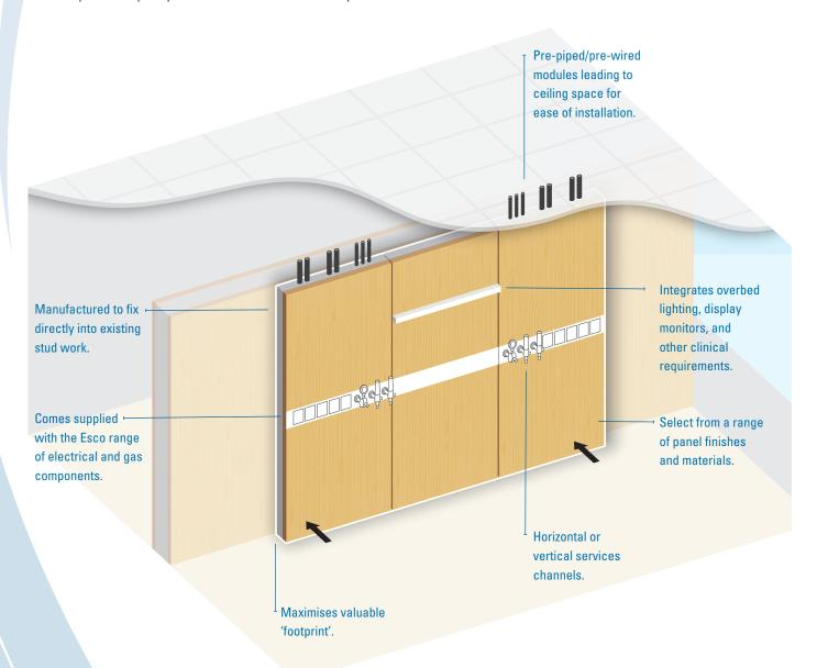
Maintaining Esco's 60 year factory manufactured quality the SigmaMax Modular Service Wall is supplied pre-wired and pre-piped for ease of installation. Key features and benefits include:
